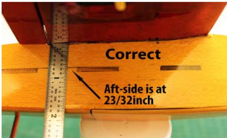
Before you glue on the wing simply raise the rear side to match or nearly match the front measurements to the center line. Here it is at  $23/32$ "
