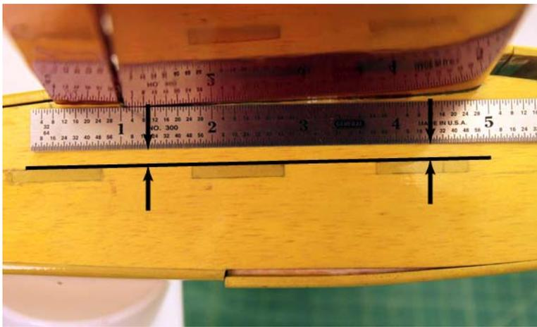
The center slots in the side of the fuselage is parallel to the True Zero Wing incidence on this plane. Therefore, you can use it as a guide to calibrate how much positive wing incidence there is on this airplane. Use a ruler to line up with the center line and you can see the front of the wing is higher than the rear side. This is positive wing incidence.
