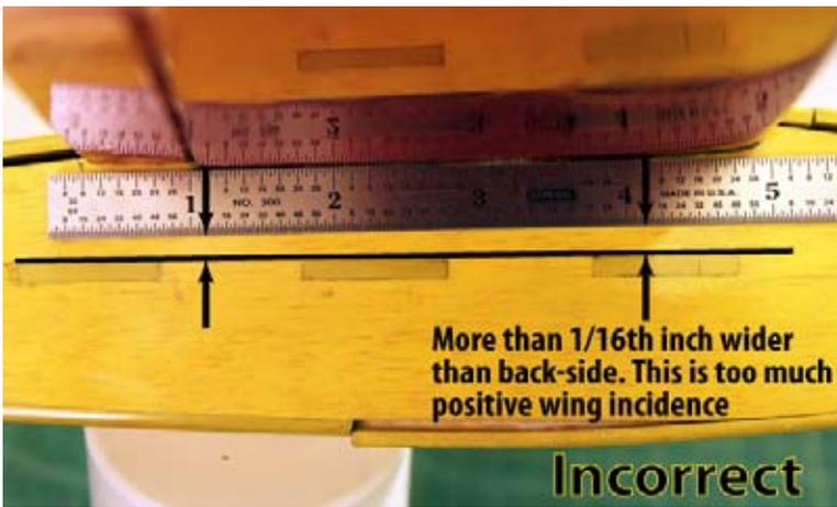
Here is another view. By aligning the ruler to the flat bottom portion of the wing you can see that there is a little over 1/16 inch positive wing incidence. This is too much and may cause the airplane to climb too much
